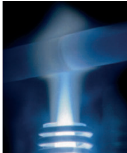
Figure 2: Production of fibre preforms via plasma outside deposition (POD)
