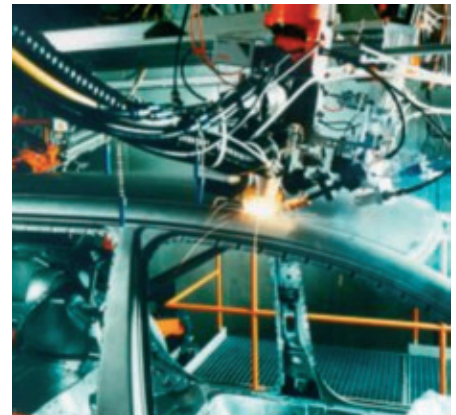
Figure 6: Materials processing, here in the automotive industry (image courtesy of Trumpf Laser GmbH & Co. KG)
